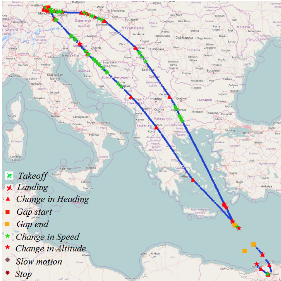
Figure 3: Types of critical points constructing the trajectory synopsis of a flying aircraft
